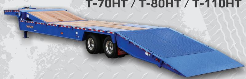
Hydraulic Tail trailers by Towmaster® are designed for the rental and construction industries. They feature a perimeter frame design, a fifth-wheel gooseneck with top deck, hydraulic folding tail, and 12,000 lb. winch. LED lights, oak wood deck, hi-tensile fabricated steel beam frame, dual parking jacks, and driver side controls are also standard. Several configurations and options are available.
