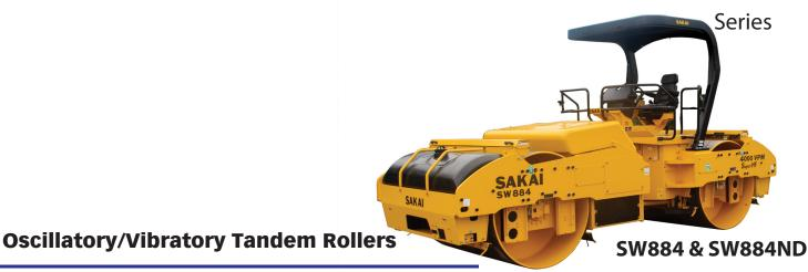
High frequency vibratory asphalt rollers are literally the fastest rollers available, featuring a high frequency of over 4,000 vpm. Designed to beat the tender zone on superpave and other perpetual pavement mixes.
