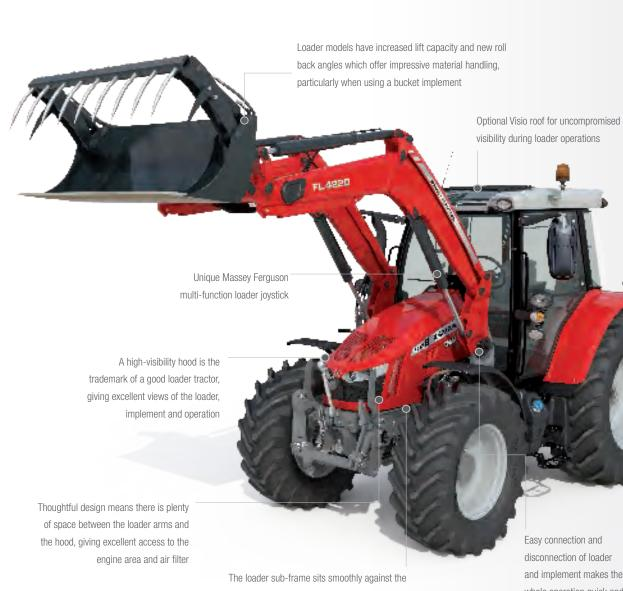
tractor chassis. Its integral structure and cast uprights have been carefully designed by our engineers who understand how a tractor and loader need to perform
