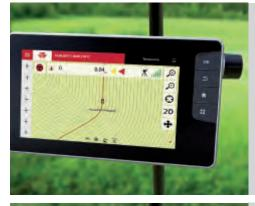
MF Guide<sup>™</sup> is Massey Ferguson's full featured, hands free steering system, available on new tractors or as an aftermarket installation for guidance ready tractors. Delivering sub-meter, decimeter and centimeter accuracy, increasing the efficiency of your farming operations saving time and money. Available with either a Trimble or Novatel receiver.
