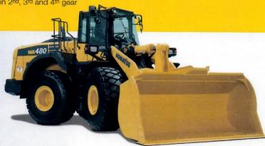
A powerful Komatsu SAA6D125E-7 engine provides a net output of 223 kW 299 HP with up to 20% improved fuel consumption.\* This engine is EPA Tier 4 Final emissions certified.
