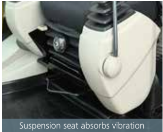
Suspension seat absorbs vibration
