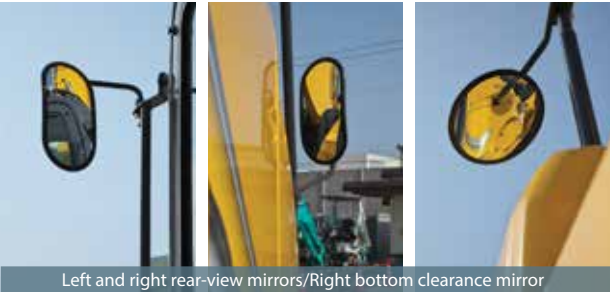
Left and right rear-view mirrors/Right bottom clearance mirror
