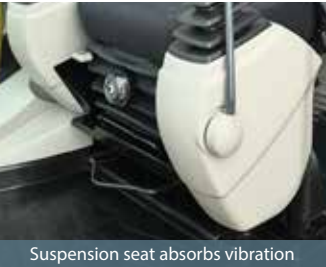
Suspension seat absorbs vibration
