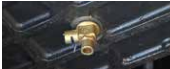
Fuel tank features bottom flange and large drain valve for easy maintenance.
