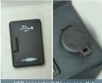
USB connector/12V power outlet
