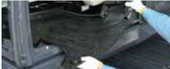
Detachable two-piece floor mat with handles for easy removal.
