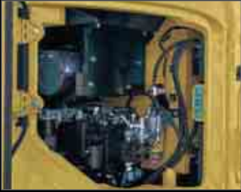
Ground level maintenance Fuel filter / Fuel filter with built-in water-separator
