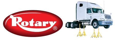
Always use safety stands when installing or removing heavy components.
