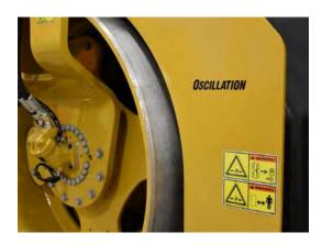
The design combines high-performance vertical vibration on the front drum with oscillation technology on the rear drum. The front drum with vertical vibration is available in two amplitude, five amplitude, or Versa-Vibe systems that provide initial compaction, while the rear drum with oscillation continues the excellent performance for optimal smoothness and density.
