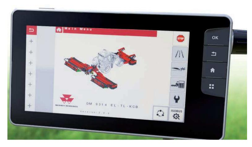
ISOBUS for total implement control – allows an implement manufacturer's control system to be displayed on the terminal screen, saving owners and operators time and money, with no need to install additional monitors in the cab. Simply plug the implement lead into the tractor's ISOBUS socket and the system automatically uploads the operating menus and displays on the screen. MF 5700 S ISOBUS conforms to the AEF (Agricultural Industry Electronic Foundation) certification.
