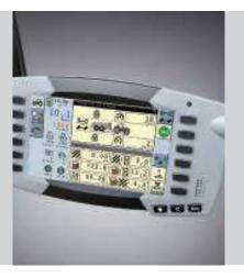
eight different memories enable the system to record information during operation on area worked, fuel use, hours worked and much more. All the settings and parameters can be stored by the terminal: A truly unique feature of C1000 is the ability to save the memorized tractor settings to a USB memory stick and manage those settings before commencing work. All these settings can be transferred between all your machines equipped with C1000.
