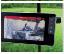
Video Mode – Pictures from an on-board camera can be displayed on the Fieldstar 5, allowing operators to monitor complex implements or simply improve safety and efficiency when reversing.
