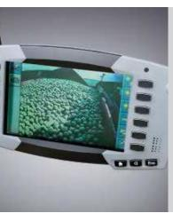
VIDEO MODE – Pictures from an onboard camera can be displayed on the console screen, allowing operators to monitor complex implements or simply improve safety and efficiency when reversing.
