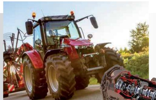
The impressive performance and deluxe design of the Dyna-4 transmission provides unbeatable productivity, control and convenience, with completely clutchless shifting of 16 forward and 16 reverse speeds.
