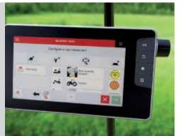
With TaskDoc all jobs' data can be recorded with minimum effort, documented in the field record and then analyzed, as applied and prescription data can be transmitted wirelessly or via USB.
