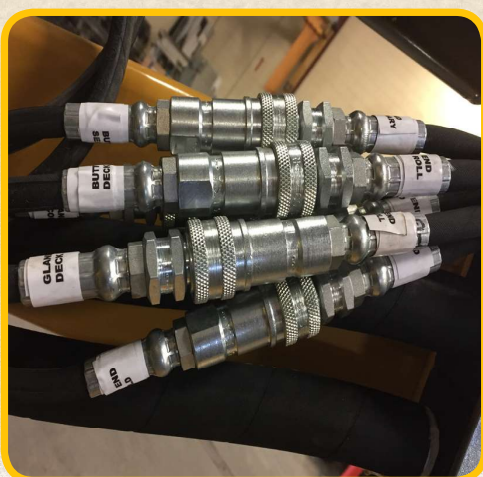
Connect 1/4" lines to matching labeled male and female ends.
