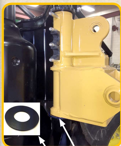
Thrust Washer goes under bottom of swivel. Part # 06520250 included.
