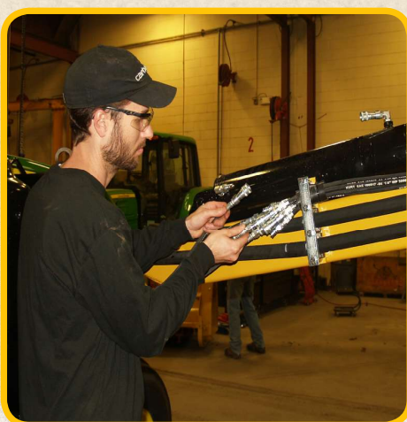
Attach 1/4" lines so that controls can be used to help lift and align boom arm with swivel pin.
