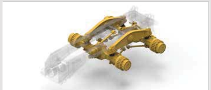
Rough terrain demands tough suspensions. Heavy-duty components absorb shocks and come back for more. You get best-in-class suspension travel and ground clearance, too.
