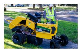
TWO-SPEED GROUND DRIVE. The operator may choose to operate in a high-range or low-range ground speed setting of 0-133 ft/min (0-40.5 m/min) to quickly move the machine or choose a slower speed when near the stump by utilizing a low-range setting of 0-66 ft/min (0-20.1 m/min).
