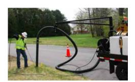
**STRONG ARM (OPTION)** With 270-degree rotation, the strong arm supports the weight of the vacuum hose and the roller head makes handling much easier by allowing smooth, fluid movements and adjustments.
