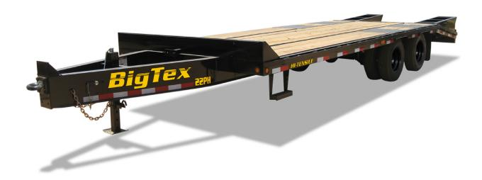
**AXLE** (2) 10,000# Dual Wheel w/ Electric Brakes (Oil
